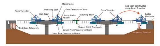
Figure 2.10: Travelling Formwork
